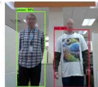
Intel Labs members demonstrate an example of artificial intelligence becoming confused by an adversarial T-shirt. (Credit: Intel Corporation)
